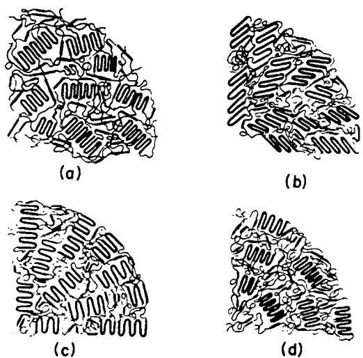
Fig. 1. Quadrants of schematic spherulite models showing different types of morphologies. After Cooper. 3
